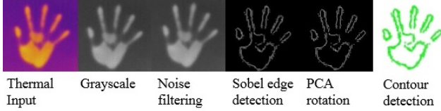
Figure 5: Feature extraction in different steps of the algorithm. The features are extracted from subject 1.
